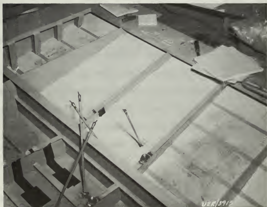
Figure III Model Showing Deflection Gages, Strain Gages, Velocity Meter Holders and ML-D2 Being Installed
